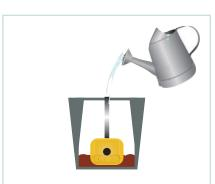
Fill the Plantsava tank with water to ensure all connections are water tight.
